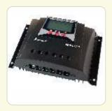
System voltage DC 12V/24V auto work Self-consumption Max 30mA Equalize charging voltage 14.6V / 29.2V Float charging voltage 13.8V/27.6V Under voltage warning protection 12V / 24V Low voltage reconnect voltage 12.5V / 25V **Terminals** 35 mm<sup>2</sup>Overload protection 37.5A/60s or 45A/5s
